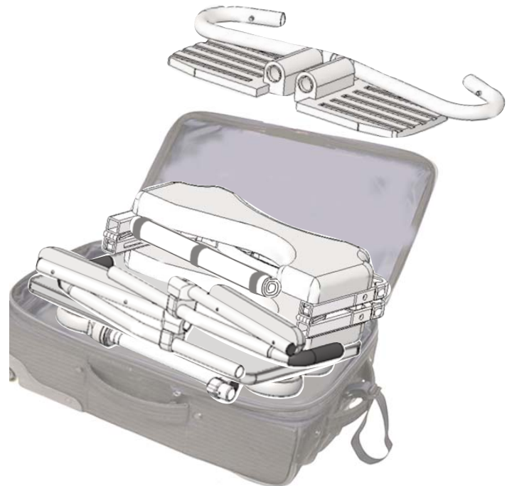
Figure D - Place the folded footrests, tools, & instructions in the zipper pouch located in the front of the carrying case.
